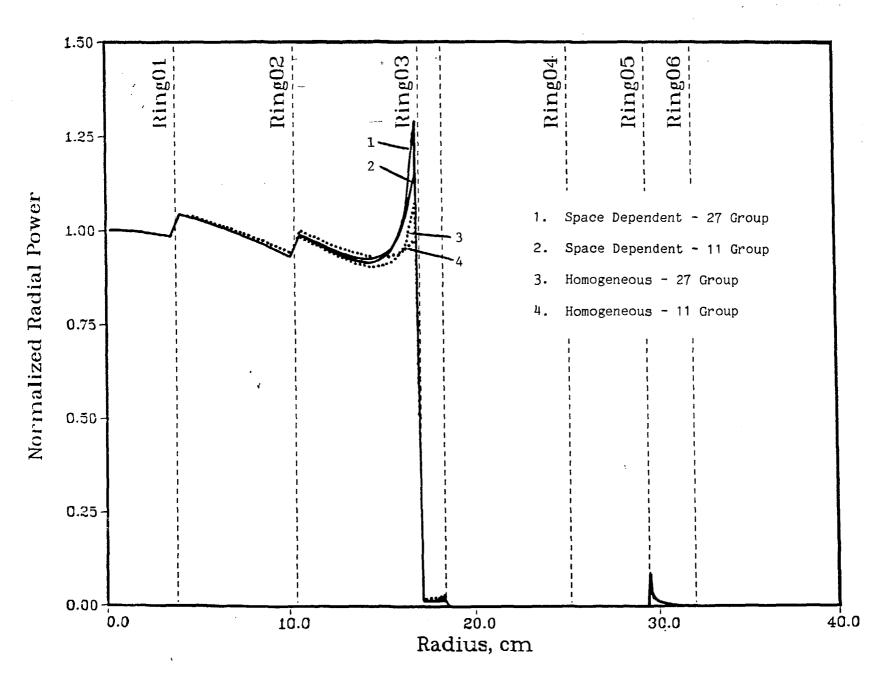
FIGURE 1. Effects of Cross Section Generation Procedure on Radial Power Distribution.
