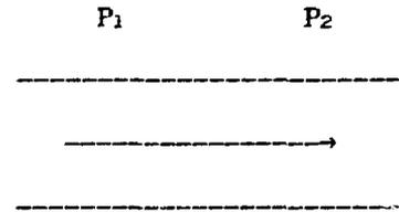
At time  $t_0 = 0$ , the velocity of the water plug contained in the pipe is assumed to be equal to zero.
