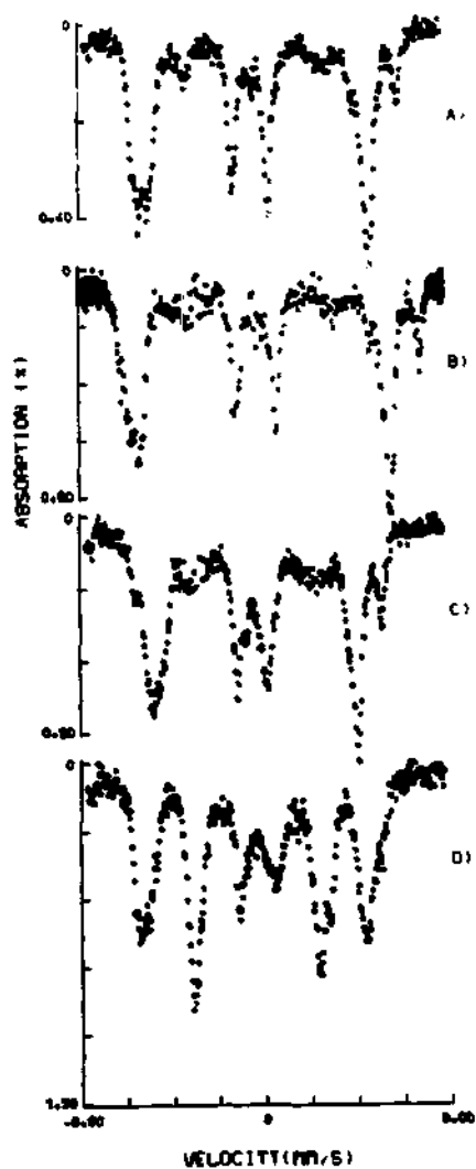
Figure 14 - ^{57}\text{Fe} Mössbauer spectra of magnetically aligned \text{Dy}_2\text{Fe}_{14}\text{B} and \text{Er}_2\text{Fe}_{14}\text{B} powder samples. Alignment at 360 K along the \gamma -propagation axis in a field of 1.7 T and freezing in paraffin/epoxy resin. Measurement of the Dy alloy at (A) 295 K, (B) 4.2 K and of the Er alloy at (C) 328 K, (D) 295 K /20/.
