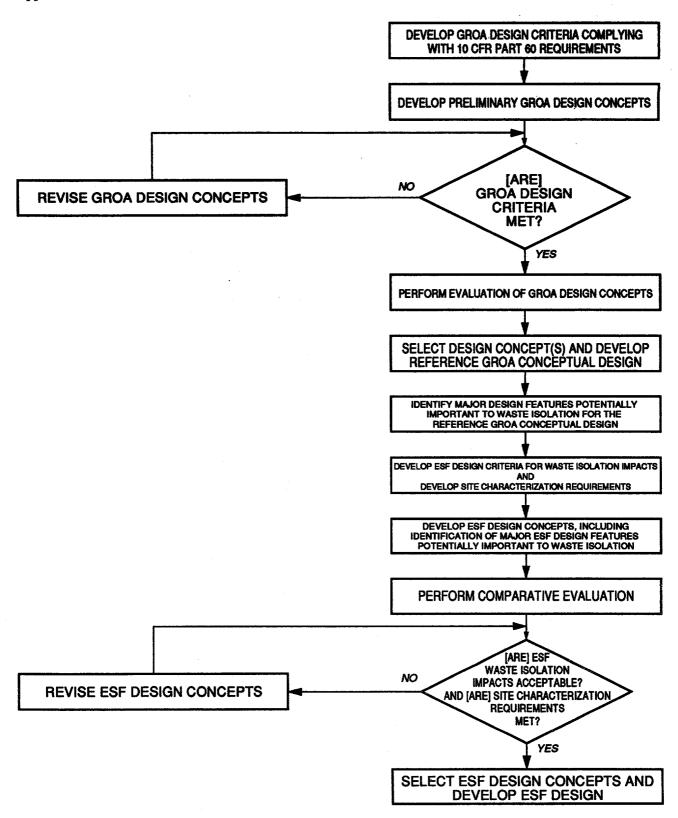
FIGURE D1 -- DOE-proposed example of an acceptable approach to achieve compliance of the ESF design with 10 CFR Part 60 requirements.
