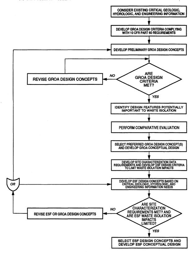
FIGURE 1 -- An example of an acceptable approach to achieve compliance of the ESF design with 10 CFR Part 60 requirements. Refer to the text in Section 4.0 (Technical Position No. 1) for a discussion of this approach.
