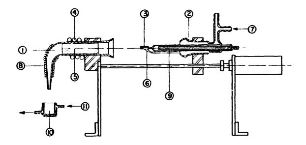
FIG.1 - Schematic diagram of remotely controlled automated apparatus for dry distillation of radioiodine from irradiated  $\text{TeO}_2$  target: 1. Outer quartz tube (fixed). 2. Inner quartz tube (movable). 3. Platinum support with  $\text{TeO}_2$ . 4. Induction coil. 5. Pt tube  $\emptyset = 22\text{mm}$ . 6. Thermo couple. 7.  $\text{O}_2\text{flow}$  (30-40ml/min). 8.Heating ribbon. 9. Electrical resistance. 10. NaOH solution. 11. Cooling liquid circulation.
