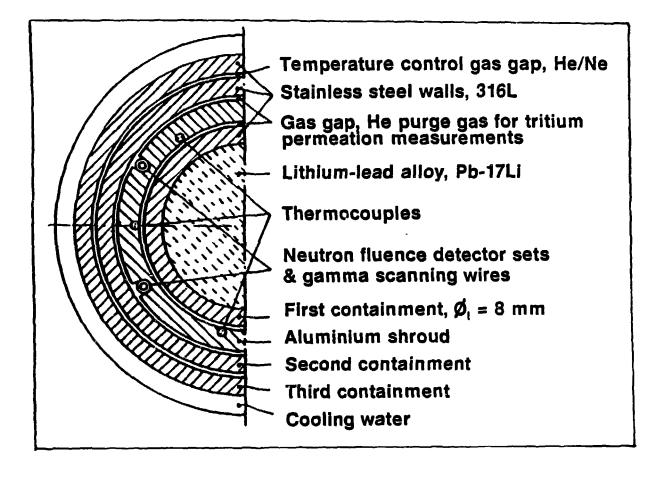
Figure 1: Cross Section of a Typical Libretto Irradiation Device
