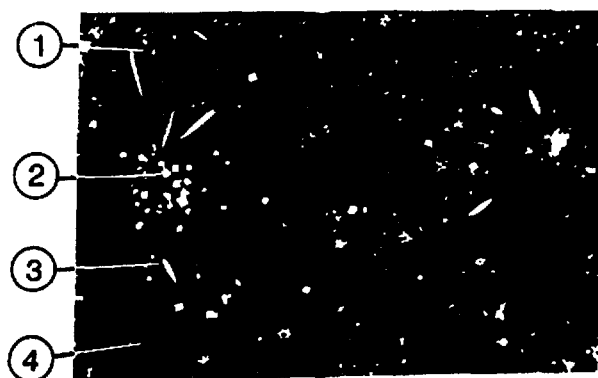
Figure 3. Crystalline Phases in Heat-Treated Glass ( \times 1300 )
