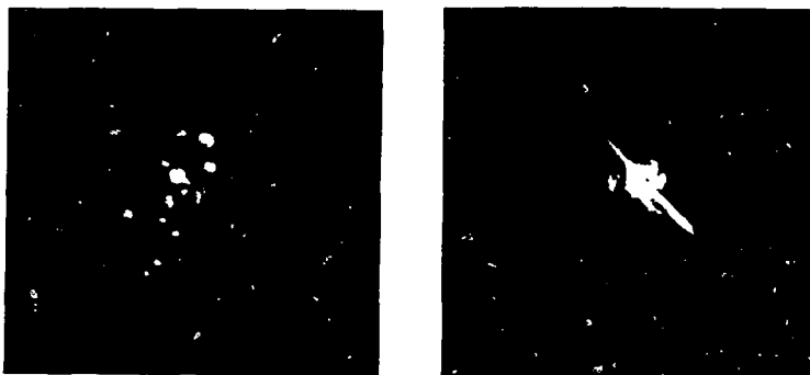
Fig. 4. Typical major bulk damage morphologies. At the left, pinpoints of damage, usually \leq 10 \mu\text{m} in size, degenerated to a "smoke trail" through the bulk material. At the right, a large damage cluster formed with one or two fractures up to 300 \mu\text{m} in length.
