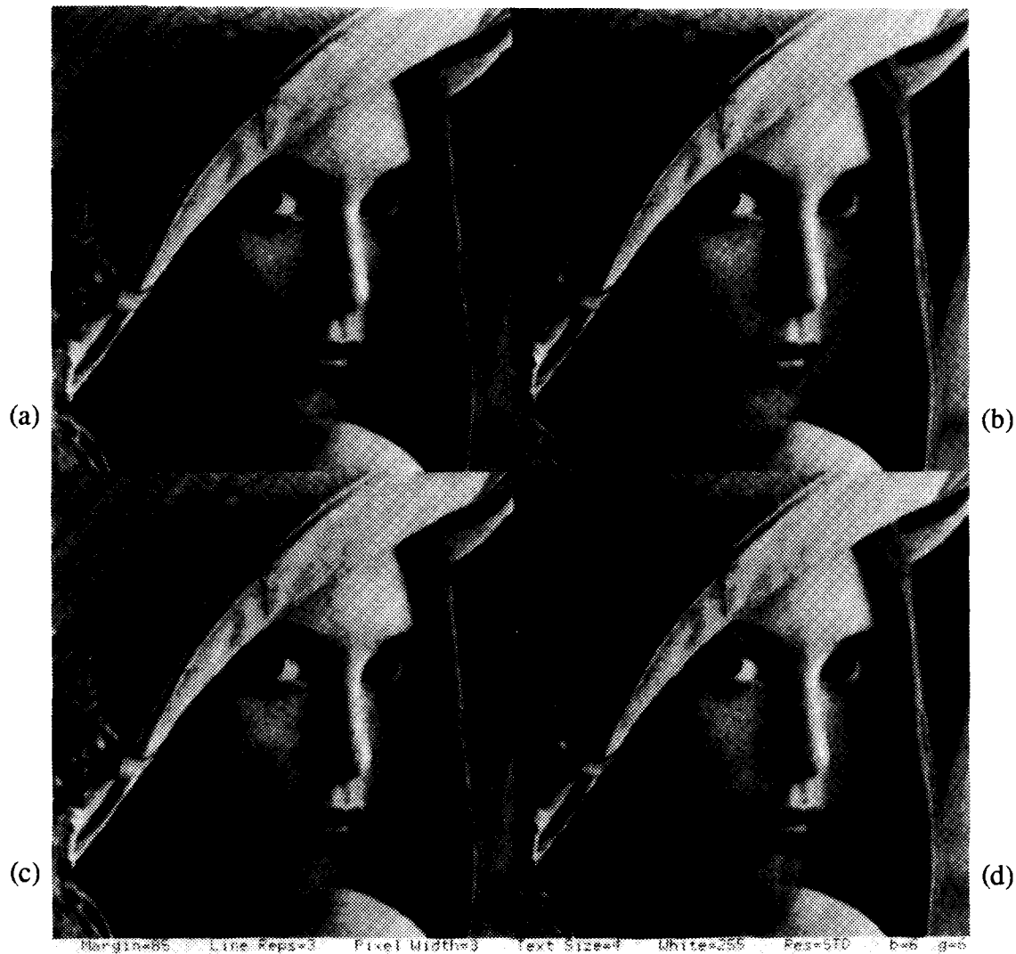
Figure 27 Simulation results on the test image Lena: (a) original image 256 \times 256 pixels, 8-bit value per pixel; (b) reconstructed with finite precision of 8 bits, PSNR = 39.3 dB; (c) compressed 8 : 1, floating points, PSNR = 32.26 dB; (d) compressed 8 : 1, 8-bit precision, PSNR = 29.02 dB.
