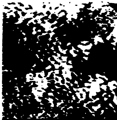
Fig. 6 STM image of an annealed Pt-DLN film (sample A). Total z-variation \approx 5 \text{ \AA} .
