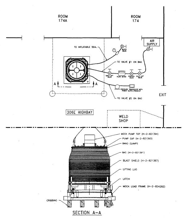
Figure 2. FRS Air Leak Test Setup at the 306E Facility
