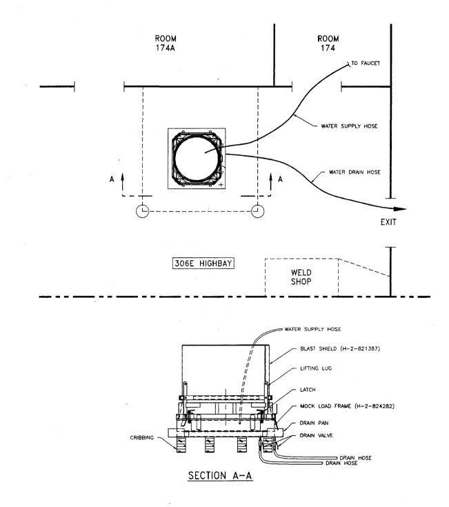
Figure 1. Blast Shield Water Leak Test Setup at the 306E Facility
