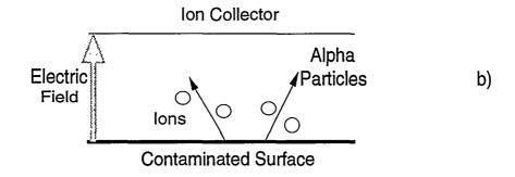
Fig. 1. Two types of LRAD-based alpha particle detection. In both cases, ions generated by alpha decays are transported to an ion collector. In an airflow sensor (a), the ions are transported to the ion collector by an air current. In an electrostatic sensor (b), the ions are transported by an electric field between the ion collector and the surface being monitored.
