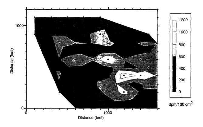
Fig. 3. Soil surface monitoring results for gross alpha contamination at a soil cleanup site. The black dots represent the measurement points. The shaded contours were interpolated between the measurements.
