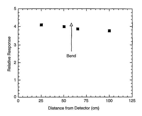
Fig. 4. Response of an alpha source placed at 4 positions in a 10-cm diameter pipe which is 125-cm long. The pipe is bent at a 90-degree angle about 60-cm from the ion detector (indicated by the arrow in the figure). Very few ions are lost in the bend.
