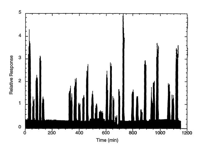
Fig. 5. Response of an airflow LRAD monitor mounted on one port in a glovebox mock-up. A large (~125,000 dpm) alpha source was placed in many different locations in the mock-up. Although the sensitivity varies, the signal is never lost in the noise.
