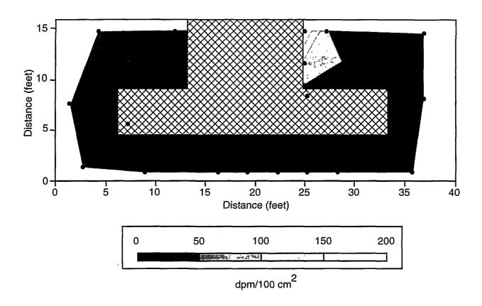
Fig. 2. Contour plot of contamination on the floor of Building 146 at TA-21 in Los Alamos. The cross-hatched area represents machines and storage covering the floor. Measurement were made at the black dots; the shaded contours were interpolated between the measurements.
