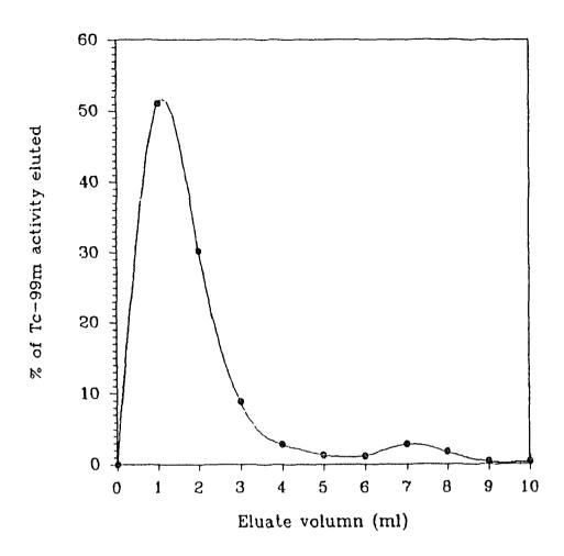
Fig. 1 Elution profile of ZrMo gel generator (flowrate 1 ml/min,wt. of gel 2 g.)
