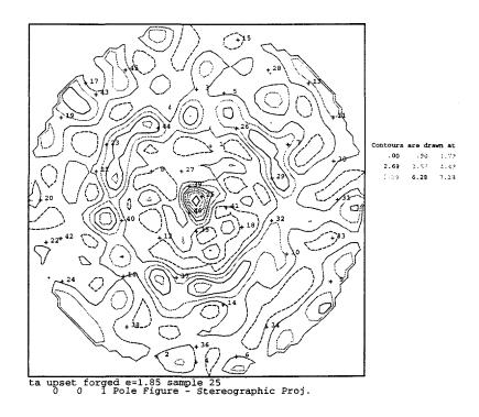
Figure 1. The (100) pole figure computed from 205 spherical harmonic coefficients ietermined via Rietveld refinement with 46 neutron TOF neutron powder diffraction patterns.
