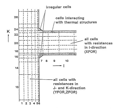
Figure 2. Input Sample Detail. Junction of Cold Leg and Downcomer.
