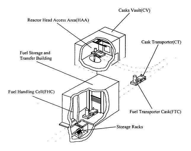
Figure 13 Reactor Refueling System(RRS)
