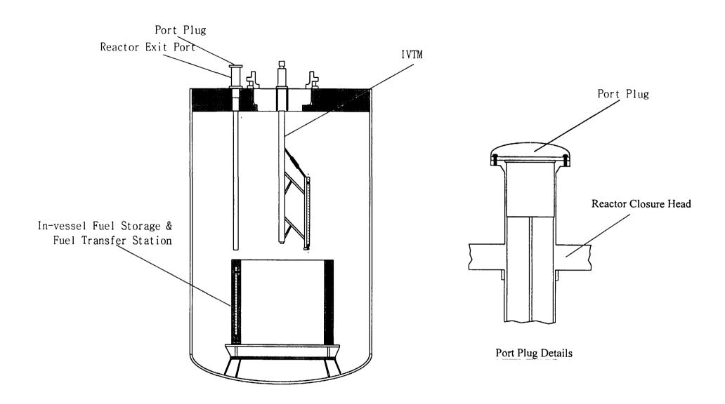
Figure 18 Fuel Transfer Port & Fuel Transfer Station
