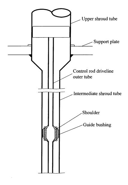
Figure 4 Upper Shroud Tube Details
