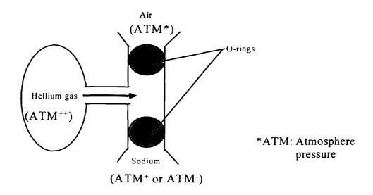
Figure 8 Buffer Seal
