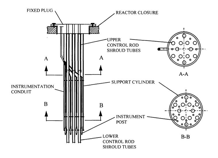
Figure 2 Upper Internal Structure
