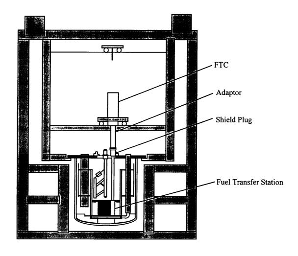
Figure 14 Section View of Reactor Refueling
