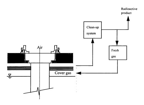
Figure 12 Conceptual diagram of Cover Gas Clean-up System
