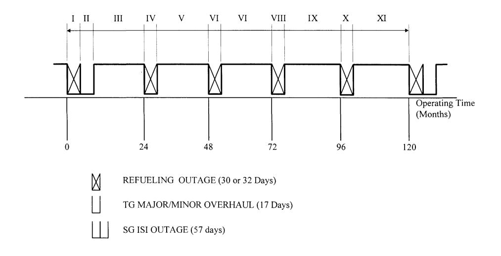
Figure 25 Operating Scenario for One Power Block
