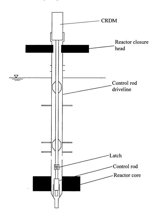
Figure 3 Section view of shroud tube and control rod
