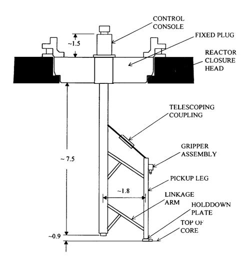
Figure 17 In-Vessel Fuel Transfer Machine (to be updated)
