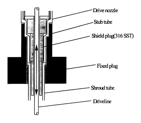
Figure 11 Shield Plug
