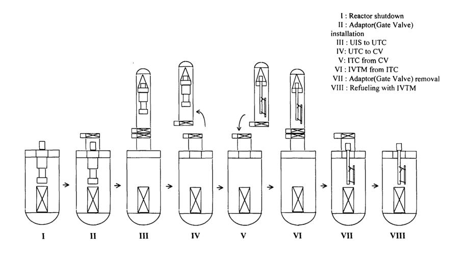
Figure 16 Conceptual Diagram of Plug-out/plug-in of the UIS System and IVTM Assembly
