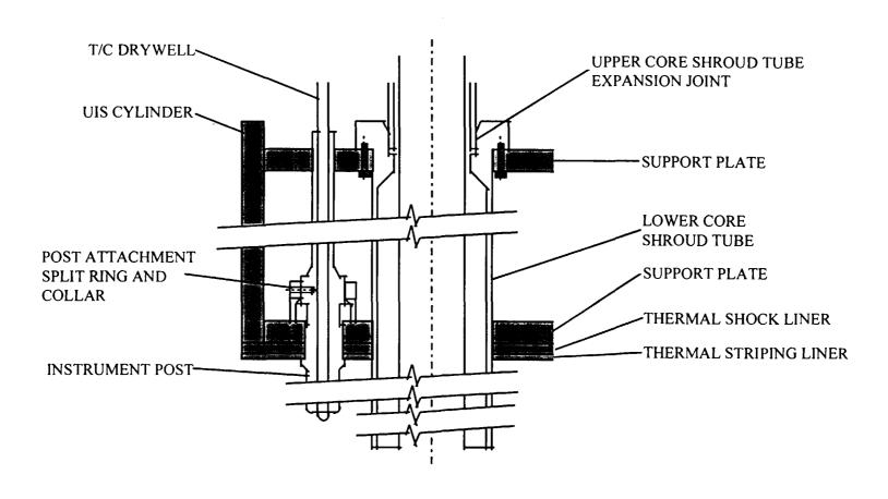
Figure 5 Upper Internal Structure Detail
