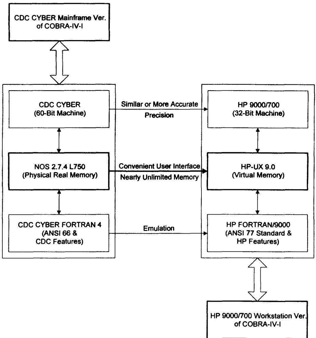
Fig. 5.1 Comparison of Features for Two Versions of COBRA-IV-I
