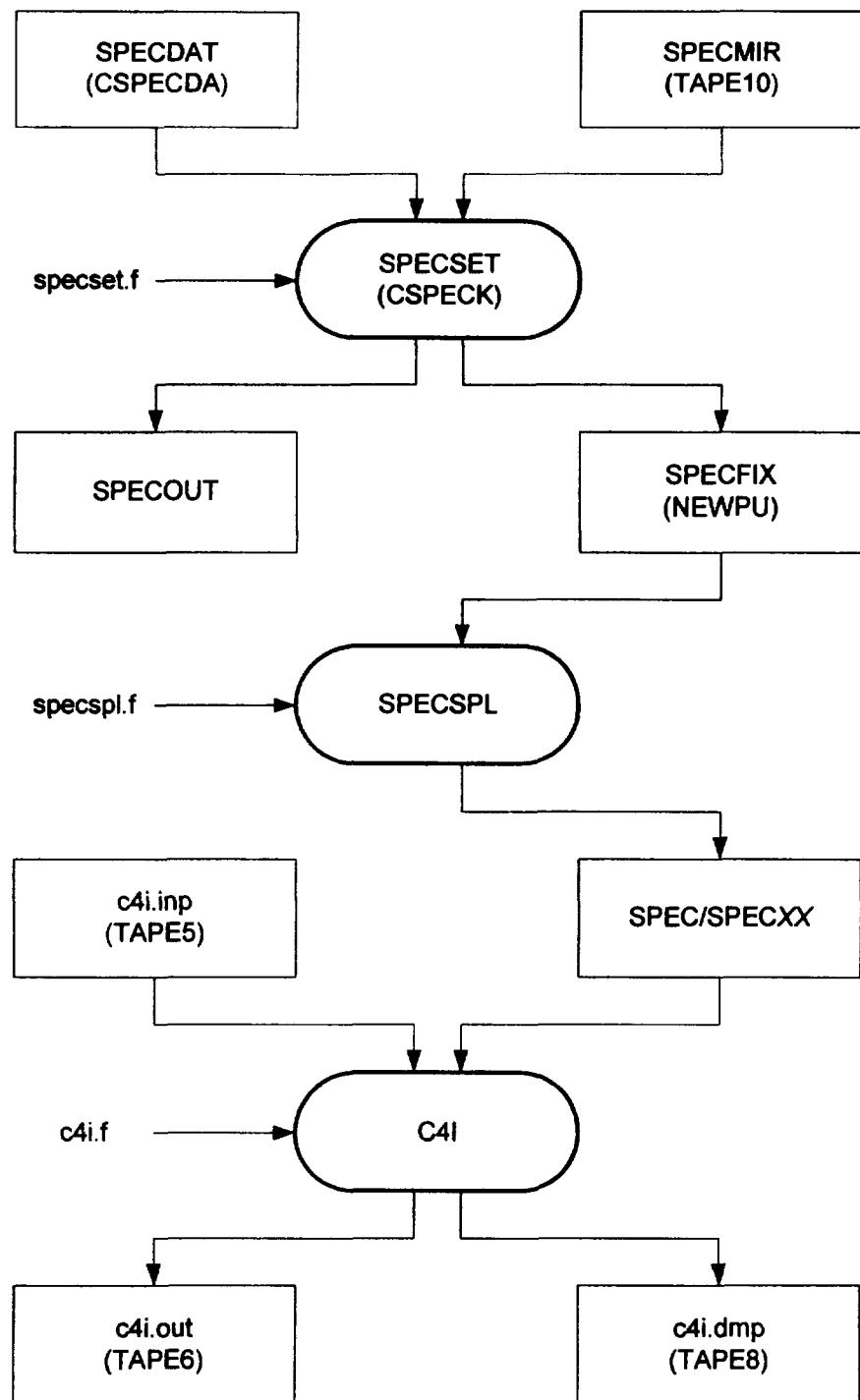
Fig. 3.1 Calculation Procedure by HP 9000/700 Version of COBRA-IV-I
