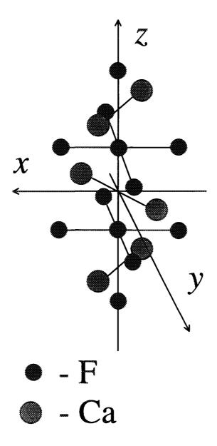
Fig. 1. Quantum cluster used in calculations.
