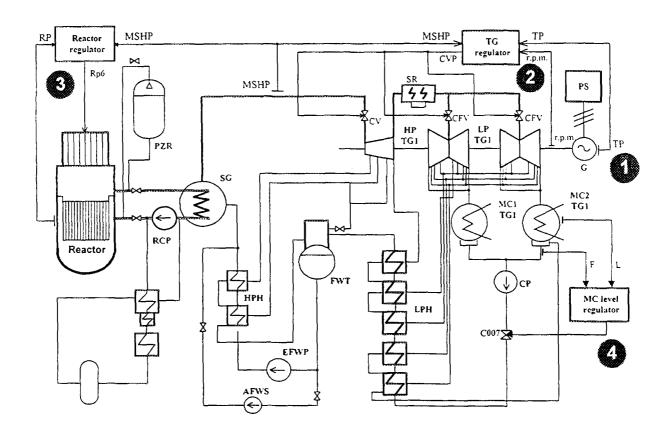
Fig. 1 Principal diagram of Dukovany NPP unit with controllers and identification of modifications for island operation mode
