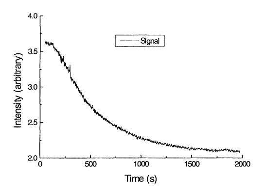
Figure 1: A typical FRS decay curve for diacetyl in pMMA,  $D_{DA} = 8 \times 10^{-15} \text{ dm}^2 \text{s}^{-1}$ .
