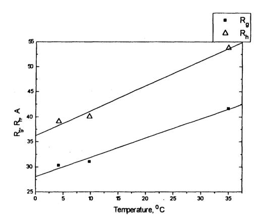
Fig. The linear dependence with the temperature of the radius of gyration,  $R_g$  (a) and of the hydrodynamic radius,  $R_h$  (b) of the 1%  $CoFe_2O_4$  particle volume concentration benzene based magnetic liquid
