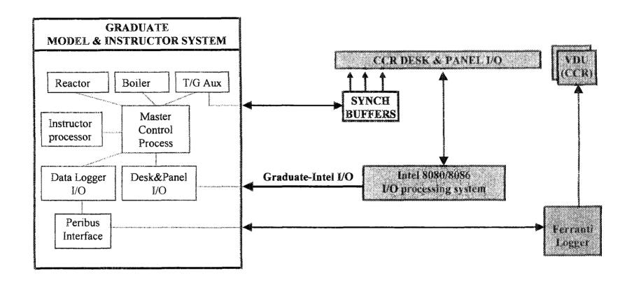
FIGURE 1 – GRADUATE/INTEL SIMULATOR ARCHITECTURE (BLOCK DIAGRAM)
