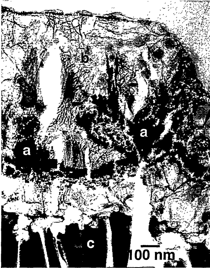
Figure 1. A TEM micrograph showing the alteration layer formed after a 14-day vapor hydration test. Visible are a) plutonium -silicate alteration crystals, b) amorphous aluminosilicate, and c) unaltered glass.
