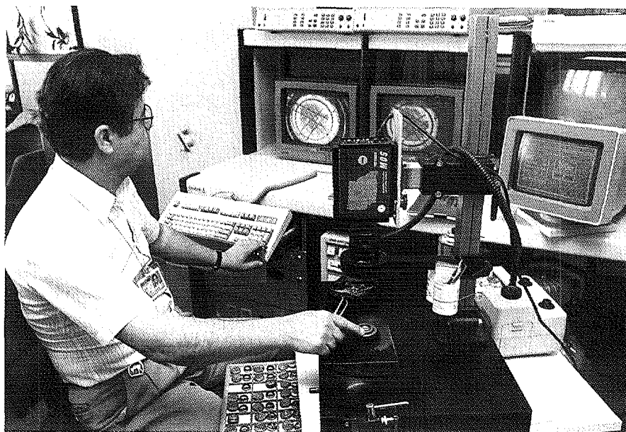
Figure 20 Comparison of metal cap seal images for seal validation.
