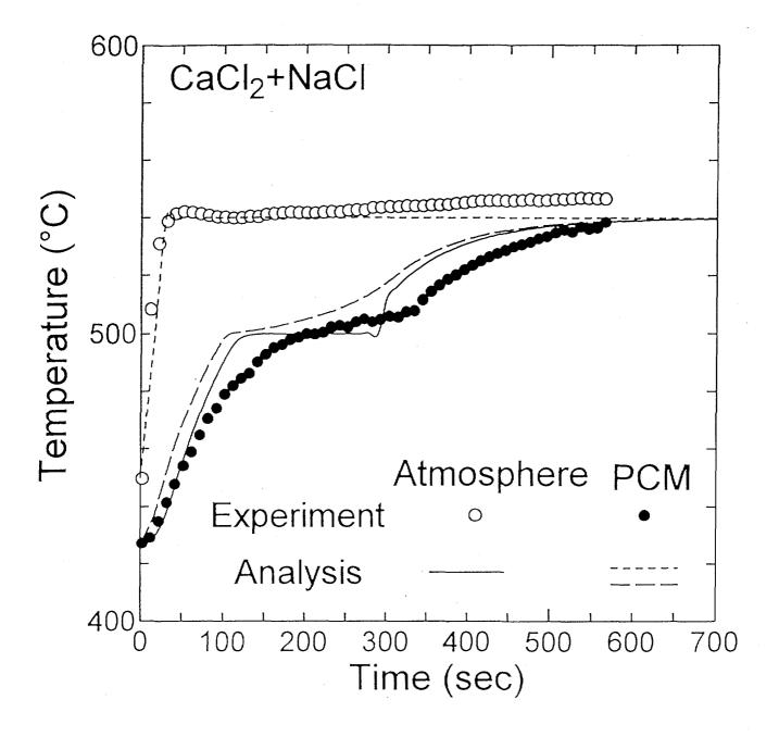
Fig. 4-8 Plot of temperature against time during melting for a porous ZrO<sub>2</sub> containing CaCl<sub>2</sub>+NaCl
