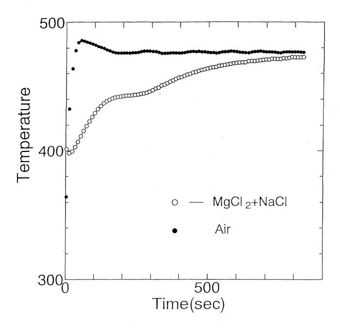
Fig. 4-6 Plot of temperature against time during melting for a porous ZrO<sub>2</sub> containing MgCl<sub>2</sub>+NaCl
