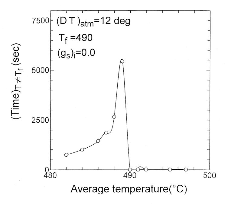
Fig. 4-17 Plot of time at which ceramic temperature begin to shift from T=Tf when atmospheric temperature varies periodically
