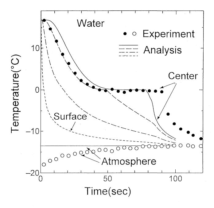
Fig. 4-3 Plot of temperature against time during solidification for a porous ZrO<sub>2</sub> containing water
