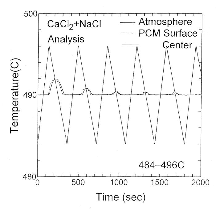
Fig. 4-14 Numerical results of temperature variations for porous ZrO<sub>2</sub> with and without PCM(CaCl<sub>2</sub>+NaCl) put in the atmosphere whose temperature is periodically changing between 484 and 496°C (initially \$s=0).
