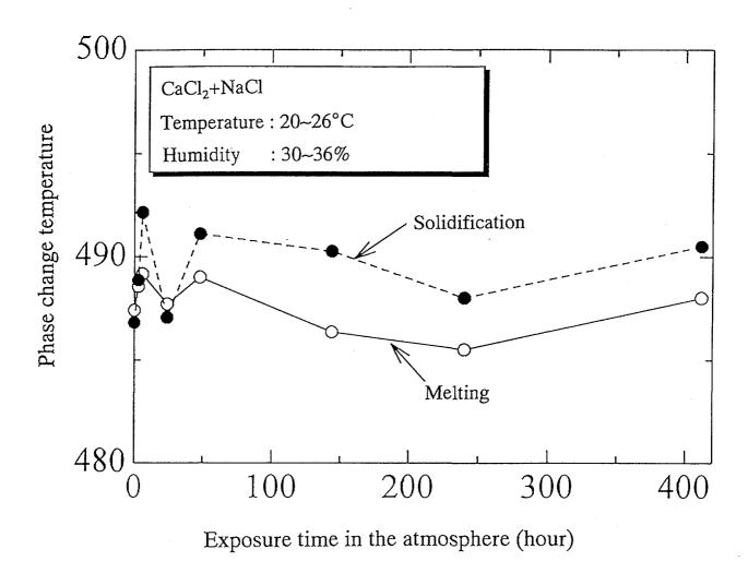
Fig. 3-14 Relation between Phase change temperature and time that molten salt was put in the atmosphere
