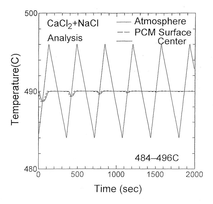
Fig. 4-15 Numerical results of temperature variations for porous ZrO<sub>2</sub> with and without PCM(CaCl<sub>2</sub>+NaCl) put in the atmosphere whose temperature is periodically changing between 484 and 496°C (initially gs=1).
