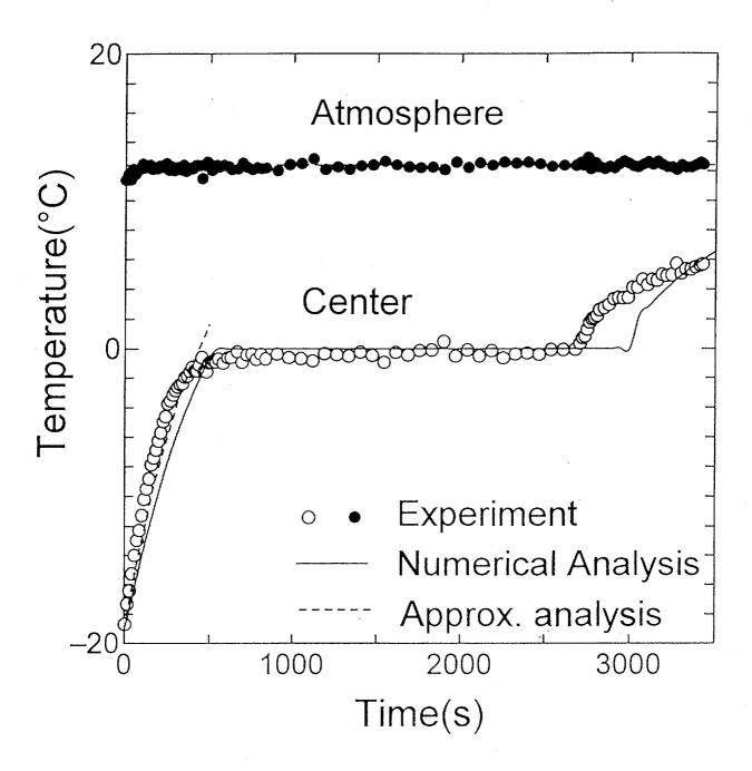
Fig. 4-2 Plot of temperature against time during melting for a porous ZrO<sub>2</sub> containing water
