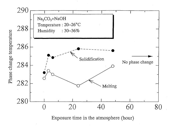
Fig. 3-6 Relation between phase change temperature and time that molten salt was put in the atmosphere
