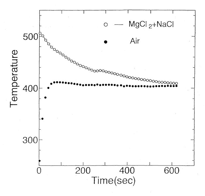
Fig. 4-7 Plot of temperature against time during solidification for a porous ZrO<sub>2</sub> containing MgCl<sub>2</sub>+NaCl
