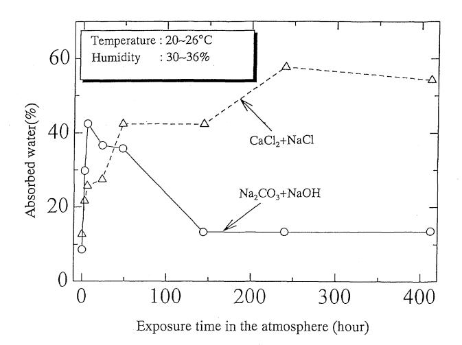
Fig. 3-7 Relation between absorbed water and time that molten salt was put in the atmosphere
