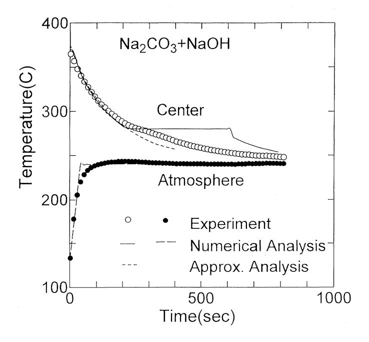
Fig. 4-5 Plot of temperature against time during solidification for a porous  $ZrO_2$  containing  $Na_2CO_3+NaOH$
