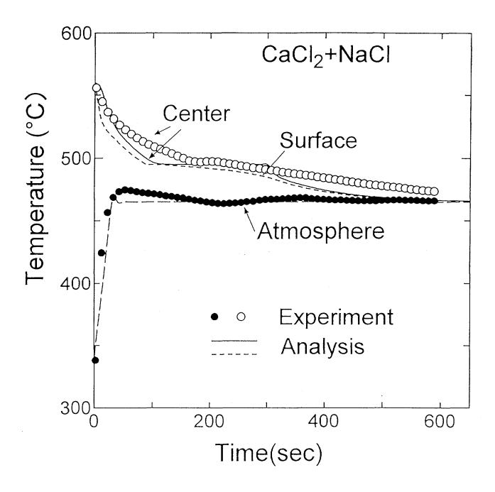
Fig. 4-9 Plot of temperature against time during solidification for a porous ZrO<sub>2</sub> containing CaCl<sub>2</sub>+NaCl
