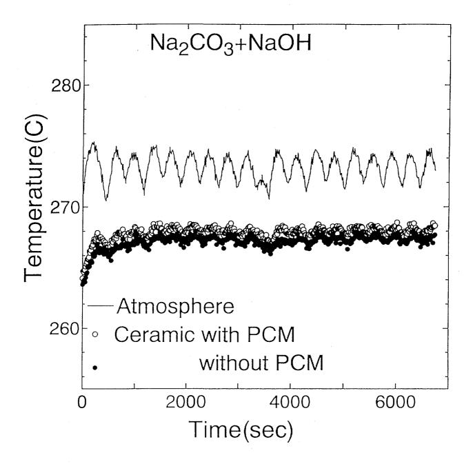
Fig. 4-10 Temperature variations of porous ZrO<sub>2</sub> with and without PCM (Na<sub>2</sub>CO<sub>3</sub>+NaOH) put in the atmosphere whose temperature is periodically changing
