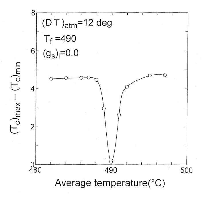
Fig. 4-16 Plot of maximum temperature difference of heat storage ceramics at steady condition against average atmospheric temperature periodically varying around the average value.
