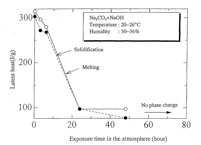
Fig.3-5 Relation between latent heat and time that molten salt was put in the atmosphere
