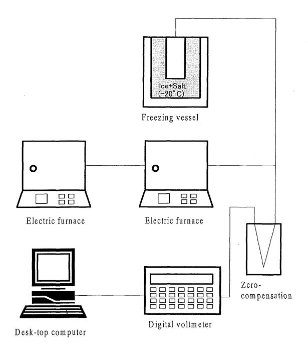
Fig. 4-1 Schematic diagram of experimental apparatus for melting and solidification
