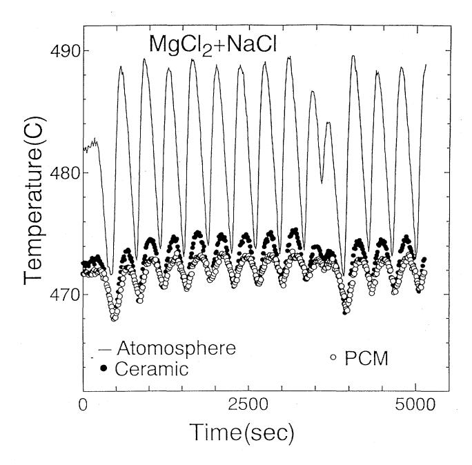
Fig. 4-11 Temperature variations of porous ZrO<sub>2</sub> with and without PCM(MgCl<sub>2</sub>+NaCl) put in the atmosphere whose temperature is periodically changing
