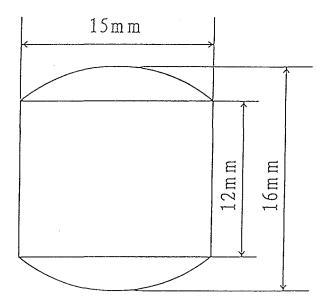
Fig. 2-1 Configuration of a ceramic material
