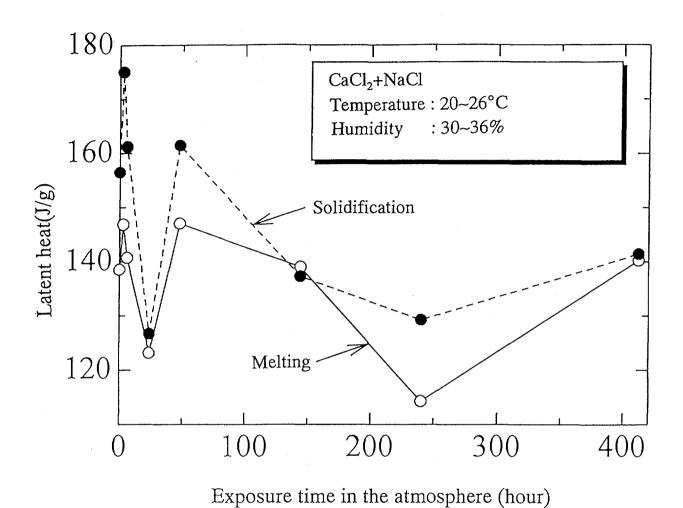
Fig. 3-13 Relation between latent heat and time that molten salt was put in the atmosphere
