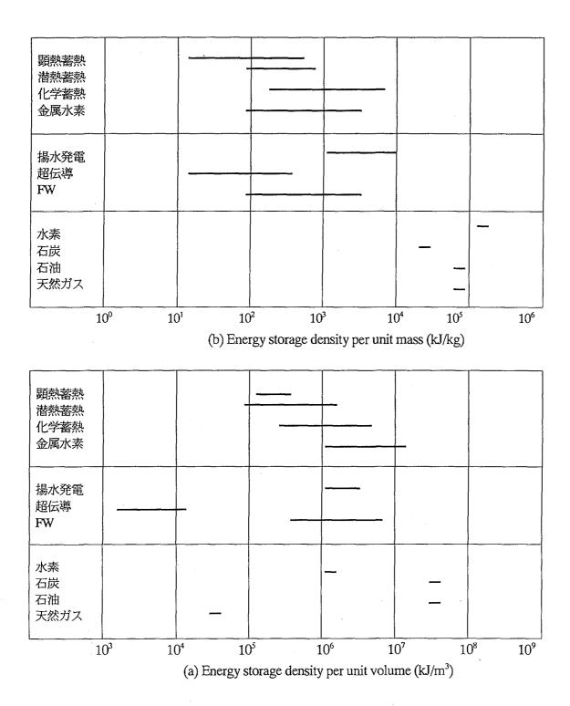
Fig. 1-1 Characteristics of several heat storage techniques and materials
