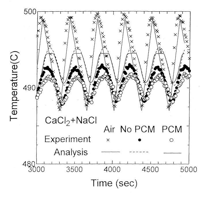
Fig. 4-12 Temperature variations of porous ZrO<sub>2</sub> with and without PCM (CaCl<sub>2</sub>+NaCl) put in the atmosphere whose temperature is periodically changing
