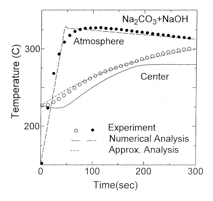
Fig. 4-4 Plot of temperature against time during melting for a porous ZrO<sub>2</sub> containing Na<sub>2</sub>CO<sub>3</sub>+NaOH
