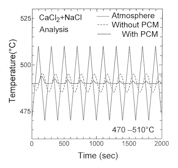
Fig. 4-13 Numerical results of temperature variations for porous ZrO<sub>2</sub> with and without PCM(CaCl<sub>2</sub>+NaCl) put in the atmosphere whose temperature is periodically changing between 470 and 510°C.
