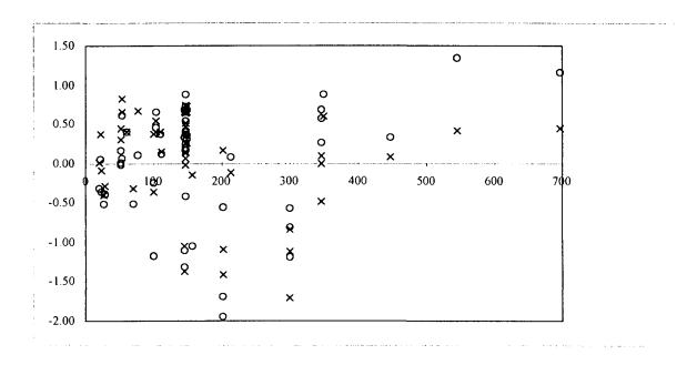
Fig. 1. Divergences between the calculation and experiment in dependence on the uranium concentration in the solution. Solution critical experiments with high-enriched uranium are considered. Circles - calculations using KENO-CONSYST; crosses - calculations using MCNP-ENDF/B-V.
