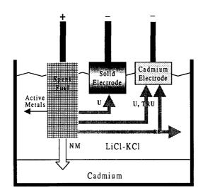
Fig. 9. Schematic representation of electrorefining process.
