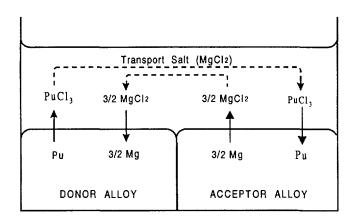
Fig. 5. Schematic representation of donor-acceptor process.
