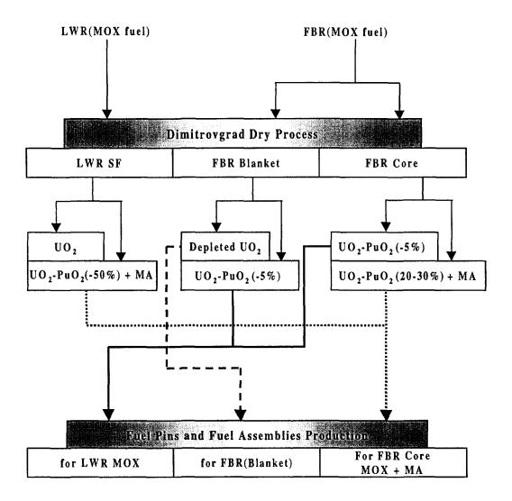
Fig. 1. UO2-PuO2 recovery method in DDP.
