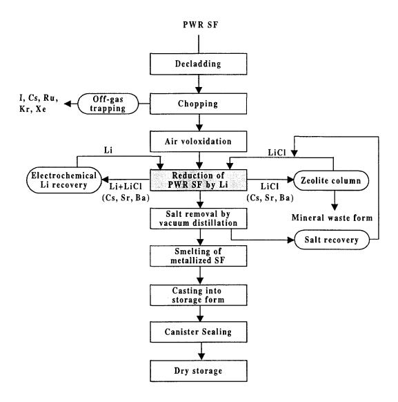
Fig. 12. Flow sheet of advanced spent fuel management process.
