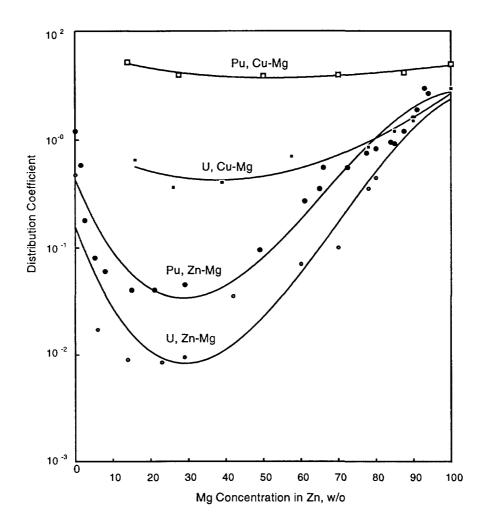
Fig. 6. Distribution of TRU elements between  $MgCl_2$  and Zn-Mg alloy.
