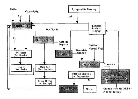
Fig. 3. Flow-sheet of  $UO_2$ -Pu $O_2$  fuel granulation process with recycled products streams.
