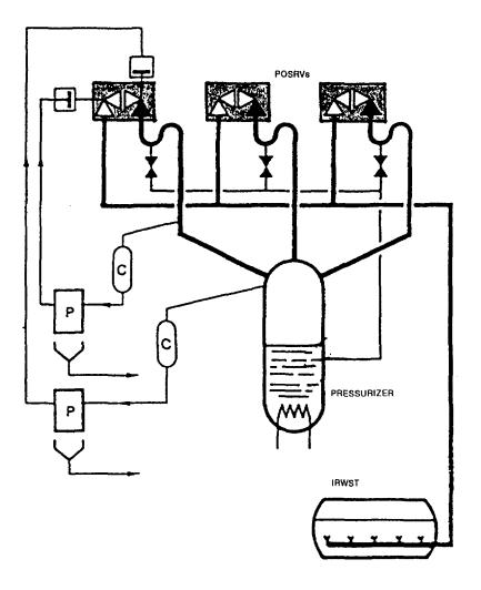
Fig. II-2. Schematic Diagram of KNGR SDS (Option 2)
