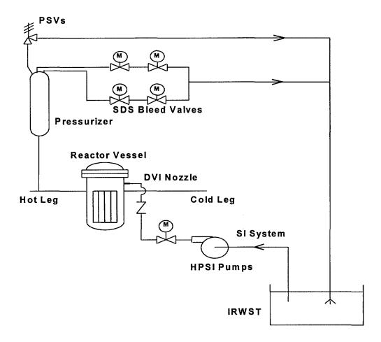
Fig. II-1. Schematic Diagram of KNGR SDS (Option 1)
