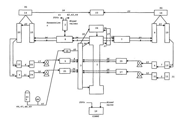
Fig. III-2. CEFLASH-4AS/REM Nodalization Scheme for TLOFW Analysis
