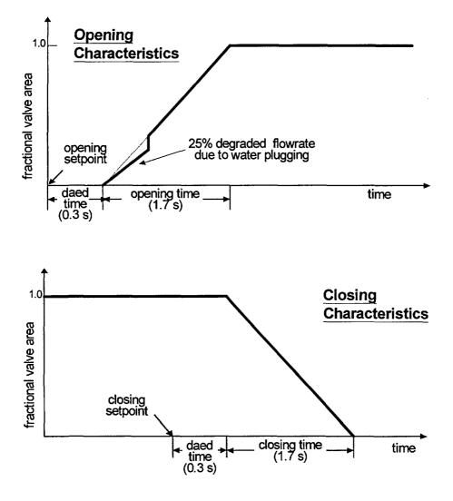
Fig. III-1. Characteristics of Sebim Valve (Option 2)
