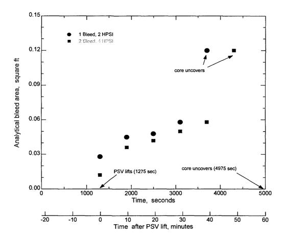
Fig. IV-7. Analytical Bleed Area Required to Prevent Core Uncovery for Various Operator Action Time (Option 1)
