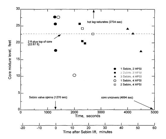
Fig. IV-13. Operator's Action Delay Time to Prevent Core Uncovery (Option
