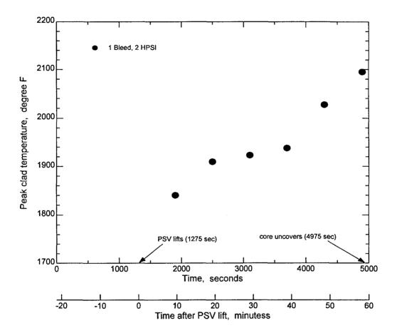
Fig. IV-8. Peak Cladding Temperature (Option 1)
