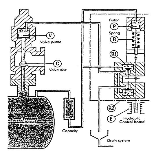
Fig. II-4. Sebim valve pilot cabinet operation
