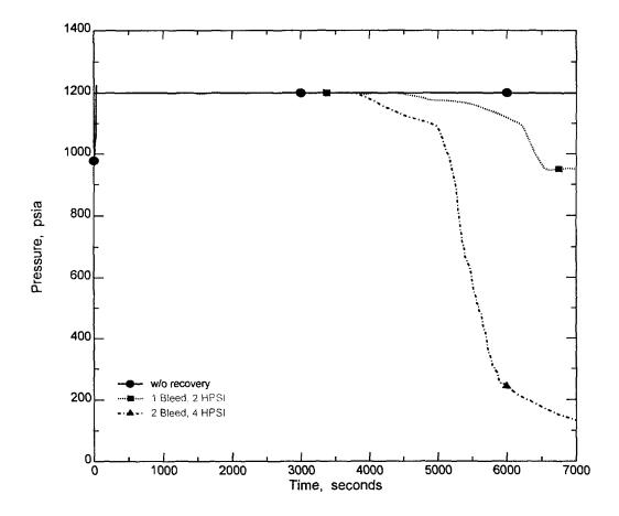
Fig. IV-3. Steam Generator Pressure (Option 1)
