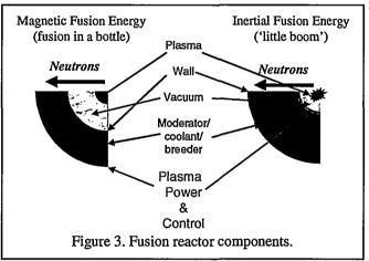
fusion reaction products. This is what I consider the hardest problem to solve for an MFE reactor. This poor wall must withstand enormous power densities and neutron irradiation without outgassing (evaporating material) significantly into the chamber. It must also survive for a long time.
