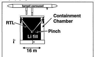
Fig.4. Sketch of a z pinch reactor chamber. [Stan - we could add a URL here for an animation of how this thing works, I have an animation and we are setting up a site.]
