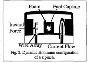
strikes the foam it generates a radiation wave and a shock. Together they move to the axis with the radiation moving faster than the shock. This radiation pushes on a capsule containing fusion fuel in the center of the imploding plasma/foam structure. If the pressure on the fuel capsule has the appropriate characteristics then the fuel will burn and a net energy release will be obtained.
