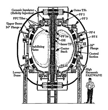
Fig.1 Partial schematic cross section of the NSTX device.
