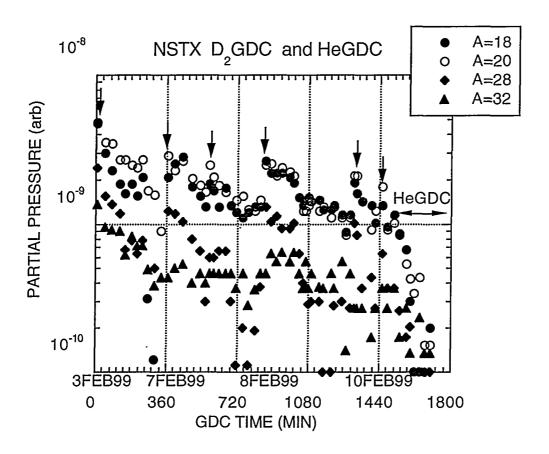
Fig.3 Comparison of  $D_2GDC$  impurity cleaning followed by HeGDC wall conditioning for February 1999 vessel configuration with few internal components. The arrows indicate the start of each  $D_2GDC$  application after a period of no GDC.  $D_2GDC$  was very effective for removing impurities from the walls. HeGDC was used to remove residual  $D_2$ .
