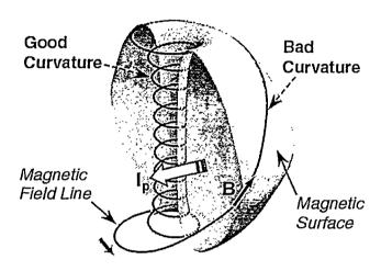
Fig.2 Schematic of Spherical Torus (ST) magnetic field line geometry.
