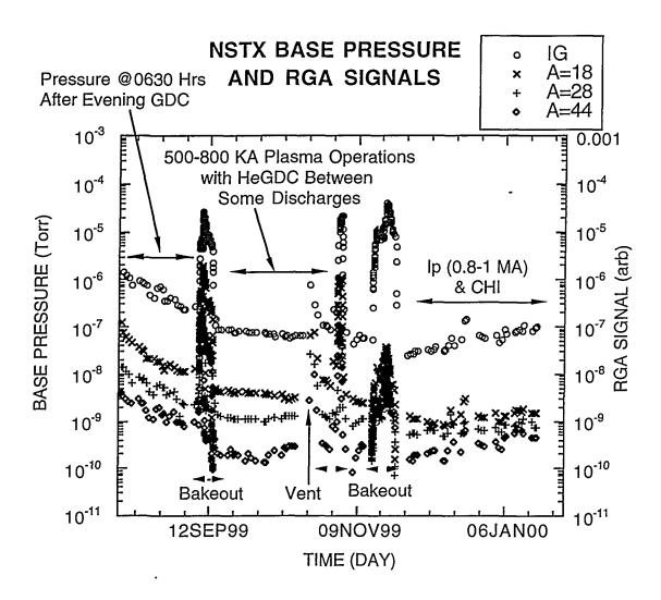
Fig.4 Vessel base pressure behavior and the partial pressures of the mass 18, 28, 32, and 44 impurity components as walls were conditioned using  $D_2GDC$ , HeGDC, and bakeout to prepare NSTX for 1 MA Discharges.
