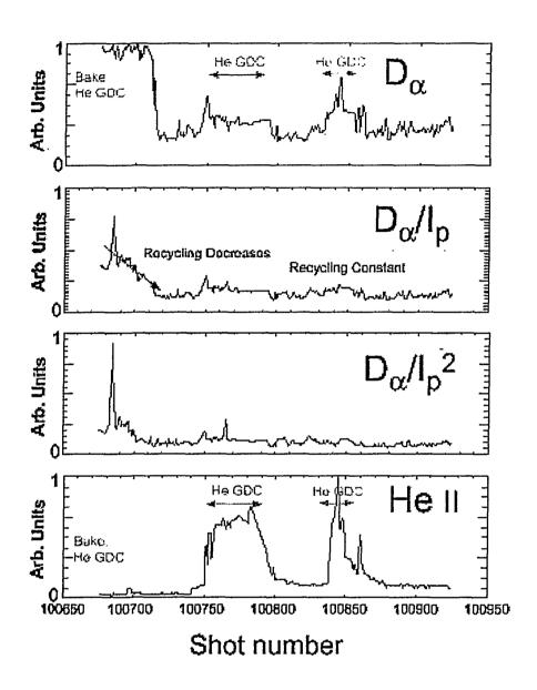
Fig.5 Edge luminousity behavior of D<sub>4</sub> and HeII for HeGDC sequences (refer to text).
