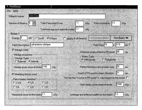
Figure 1. Input screen for beam 1 of two-beam calculation. At the top the total results are shown, at the bottom the results for beam 1
