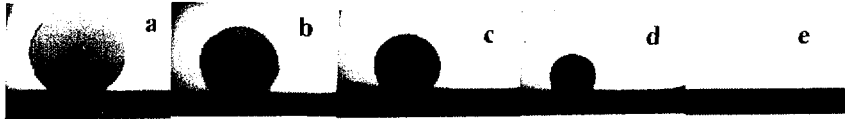
Fig. 5. The kinetics of Cu impregnation of an unsintered TiC substrate at 1150°C
