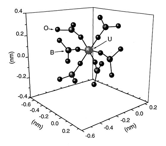
Fig. 1 Simulated local structure for uranyl in  $B_2O_3$  glass matrix.
