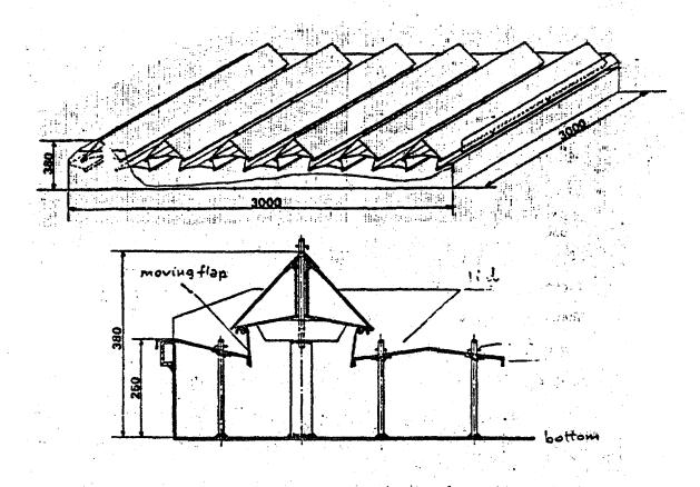
FIGURE 2: BASIC ELEMENT OF A SUFFOCATION CATCH TRAY
