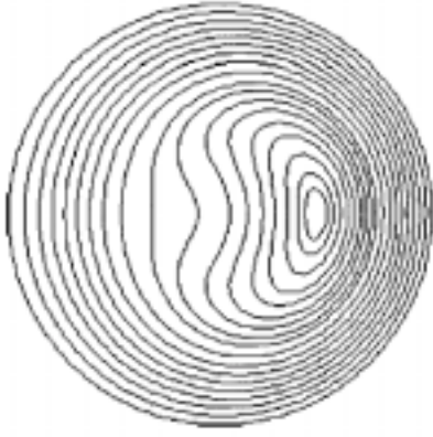
FIG. 2. Poloidal section of single helicity magnetic surfaces computed through the helical Grad-Shafranov equation and Ohm's law.
