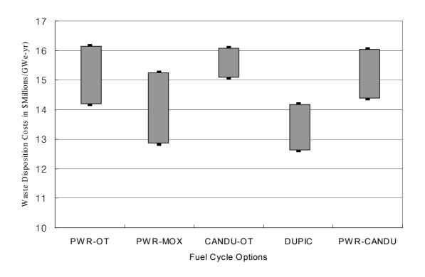
Fig. 4 Range of the Waste Management Cost for Five Fuel Cycle Options
