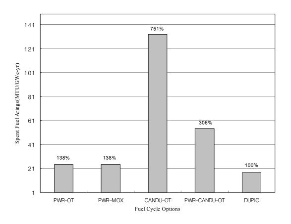
Fig. 3 Spent Fuel Arisings Comparison (Based on 1 GWe-yr)
