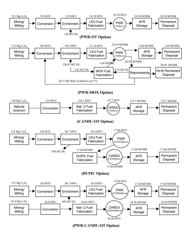
Fig. 1 Five Fuel Cycle Options and Their Material Flows (Based on 1 GWe-yr)
