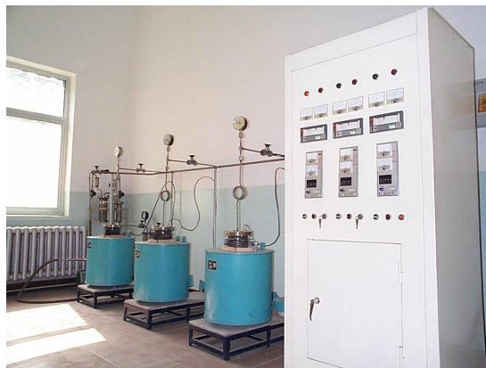
Fig. 3 W-Na compatibility test facility
