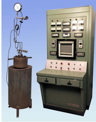
Fig. 10 Autoclave system for W-H 2 O compatibility test
