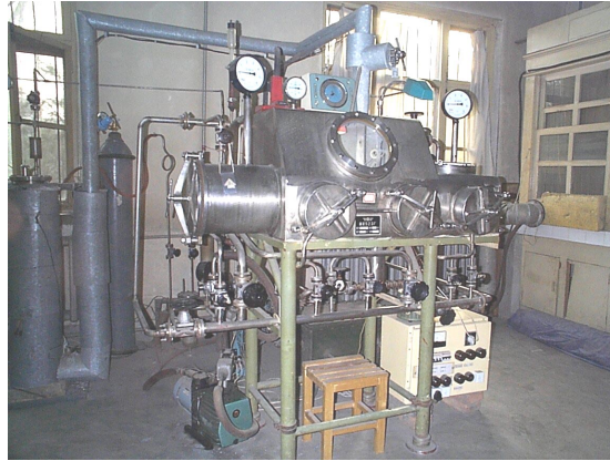
Fig. 2 Glove box system with inert gas
