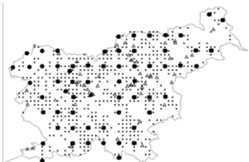
FIG. 1. A map of inventory plots ( 4 \times 4 km grid) for IAP determination (small spots), 16 \times 16 km grid for H. physodes collection (big spots) and SO_2 air measurement sampling locations (open triangle).
