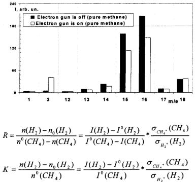
Part of pure methane mass spectrum is shown on the figure. Average energy of activating electrons was about 2,5 keV, electron current ~ 200 mA. The conversion ratios K, R were calculated. R shows number of hydrogen molecules produced by one molecule of methane spent, where n(i) is the concentration of
