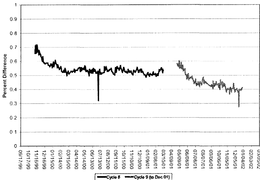
Figure 5: Unit 1 LEFM - Venturi Measurement FFW Flow Difference for Cycle 8 to and Cycle 9 to Dec. 01
