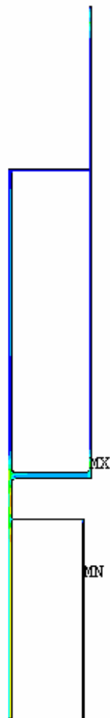
Fig. 17 Tresca stress intensity contour at time=2 hours during cool-down operation
