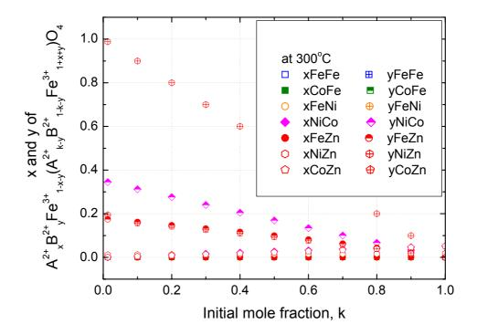
Fig. 17 The values of chemical composition, x and y, of  $A^{2^+}{}_xB^{2^+}{}_yFe^{3^+}{}_{1^-x^-y}(A^{2^+}{}_{k^-x}B^{2^+}{}_{1^-k^-y}Fe^{3^+}{}_{1^+x^+y})O_4 \ varied \ with \ initial \ mole \\ fraction \ k \ at \ 300\,{}^{\circ}{}{}^{\circ}{}^{\circ}$
