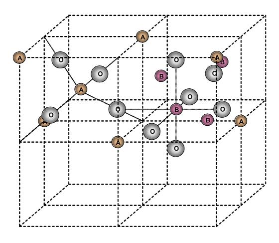
Fig. 2 A schematic diagram of the lattice structure of spinel compound
