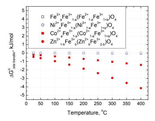
Fig. 5 The Gibbs free energy change with temperature in some spinel compounds
