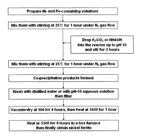
Fig. 25 Procedure for nickel ferrite synthesis by co-precipitation method
