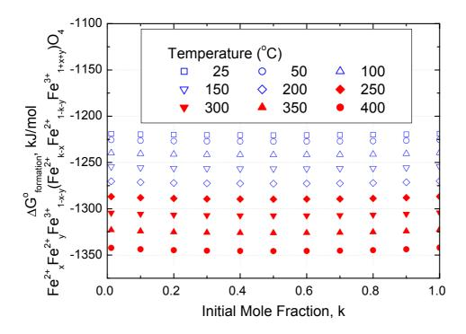
Fig. 7 The change of free energy of formation,  $\triangle G^o_{formation}$ , of  $Fe^{2^+}_{\ x}Fe^{2^+}_{\ y}Fe^{3^+}_{\ 1^-x^-y}(Fe^{2^+}_{\ k^-x}Fe^{2^+}_{\ 1^-k^-y}Fe^{3^+}_{\ 1^+x^+y})O_4$  varied with initial mole fraction k at various temperatures
