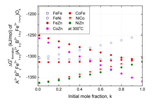
Fig. 21 The change of free energy of formation,  $\triangle G^o_{\text{formation}}$ , of  $A^{2^+}{}_xB^{2^+}{}_yFe^{3^+}{}_{1^-x^-y}(A^{2^+}{}_{k^-x}B^{2^+}{}_{1^-k^-y}Fe^{3^+}{}_{1^+x^+y})O_4 \text{ varied with initial mole fraction } k \text{ at } 300\,^{\circ}\text{C}$
