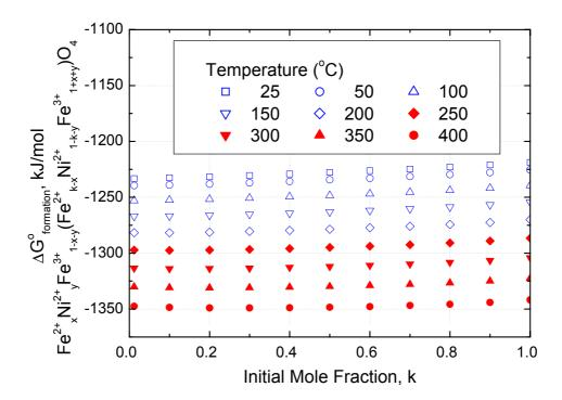
Fig. 9 The change of free energy of formation,  $\triangle G^o_{formation}$ , of  $Fe^{2^+}_{\ x}Ni^{2^+}_{\ y}Fe^{3^+}_{\ 1-x-y}(Fe^{2^+}_{\ k-x}Ni^{2^+}_{\ 1-k-y}Fe^{3^+}_{\ 1+x+y})O_4$  varied with initial mole fraction k at various temperatures
