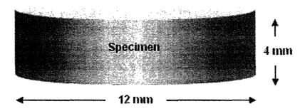
Fig. 26 The test specimen pressed under 3000 lbs for chemical analysis
