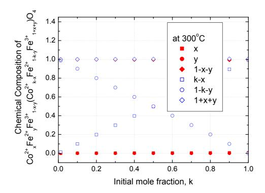
Fig. 10 The values of chemical composition, x+y, 1-x-y and 1+x+y, of  $Co^{2+}{}_xFe^{2+}{}_yFe^{3+}{}_{1-x-y}(Co^{2+}{}_{k-x}Fe^{2+}{}_{1-k-y}Fe^{3+}{}_{1+x+y})O_4 \ \ \text{varied with initial mole fraction } k \ \text{at } 300\,^{\circ}\text{C}$
