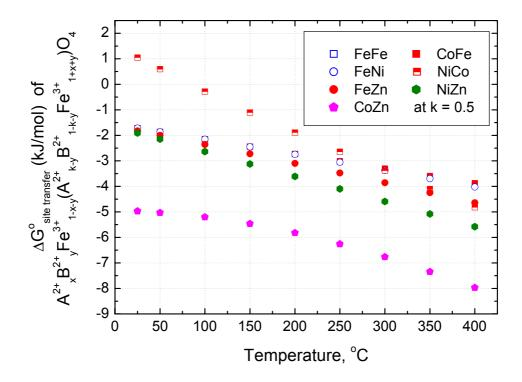
Fig. 20 The change of free energy of site transfer,  $\triangle G^o_{\text{site transfer}}$ , of  $A^{2^+}{}_xB^{2^+}{}_yFe^{3^+}{}_{1^-x^-y}(A^{2^+}{}_{k^-x}B^{2^+}{}_{1^-k^-y}Fe^{3^+}{}_{1^+x^+y})O_4 \qquad \text{varied} \qquad \text{with temperature at initial mole fraction } k=0.5$
