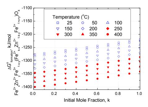
Fig. 13 The change of free energy of formation,  $\triangle G^{o}_{formation}$ , of  $Fe^{2_{+}}_{x}Zn^{2_{+}}_{y}Fe^{3_{+}}_{1-x-y}(Fe^{2_{+}}_{k-x}Zn^{2_{+}}_{1-k-y}Fe^{3_{+}}_{1+x+y})O_{4}$  varied with initial mole fraction k at various temperatures
