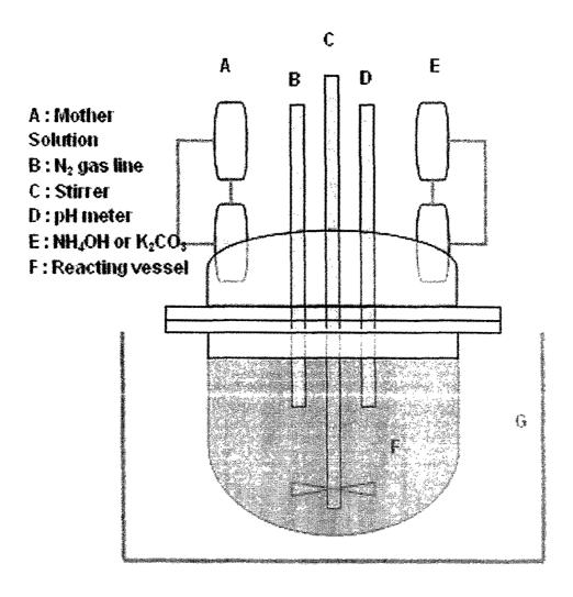
Fig. 24 Schematic diagram of an experimental apparatus for ferrite synthesis
