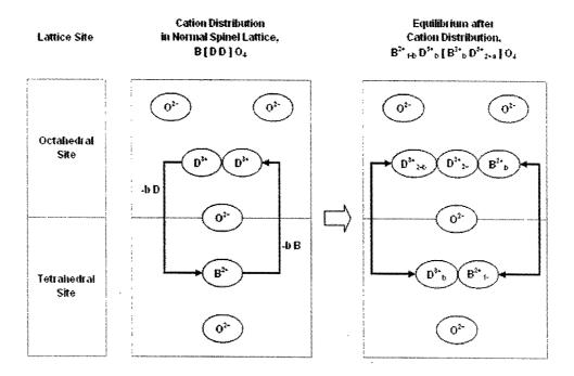
Fig. 3 Cation distribution in the lattice of inverse spinel and normal spinel
