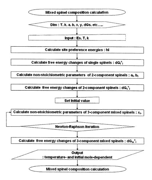
Fig. 23 Algorithm for calculation of chemical composition and free energy dependent on temperature and initial mole fraction
