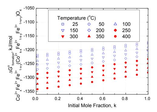
Fig. 11 The change of free energy of formation,  $\triangle G^o_{formation}$ , of  $Co^{2_+}{}_xFe^{2_+}{}_yFe^{3_+}{}_{1-x-y}(Co^{2_+}{}_{k-x}Fe^{2_+}{}_{1-k-y}Fe^{3_+}{}_{1+x+y})O_4$  varied with initial mole fraction k at various temperatures
