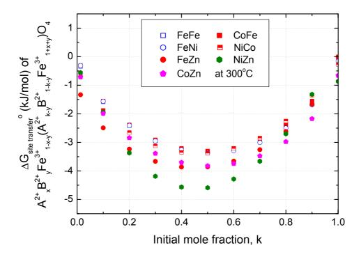
Fig. 19 The change of free energy of site transfer,  $\triangle G^o_{\text{site transfer}}$ , of  $A^{2^+}{}_x B^{2^+}{}_y F e^{3^+}{}_{1^-x^-y} (A^{2^+}{}_{k^-x} B^{2^+}{}_{1^-k^-y} F e^{3^+}{}_{1^+x^+y}) O_4 \text{ varied with initial mole}$  fraction k at 300°C
