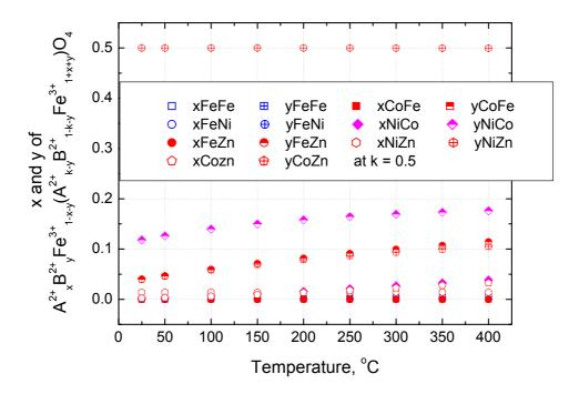
Fig. 18 The values of chemical composition, x and y, of  $A^{2^+}{}_xB^{2^+}{}_y$   $Fe^{3^+}{}_{1^-x^-y}(A^{2^+}{}_{k^-x}B^{2^+}{}_{1^-k^-y}Fe^{3^+}{}_{1^+x^+y})O_4 \quad \text{varied} \quad \text{with temperature at initial mole fraction } k=0.5$
