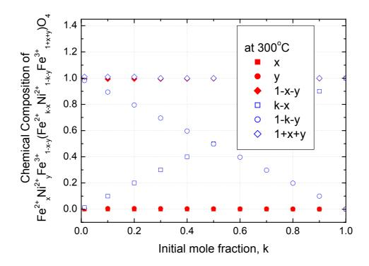
Fig. 8 The values of chemical composition, x+y, 1-x-y and 1+x+y, of  $Fe^{2^+}{}_xNi^{2^+}{}_yFe^{3^+}{}_{1-x-y}(Fe^{2^+}{}_{k-x}Ni^{2^+}{}_{1-k-y}Fe^{3^+}{}_{1+x+y})O_4 \ \ varied \ \ with \ \ initial mole fraction k at 300 °C$
