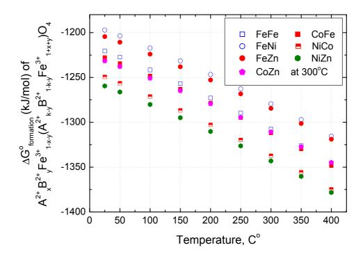
Fig. 22 The change of free energy of formation,  $\triangle G^o_{\text{formation}}$ , of  $A^{2^+}_{x}B^{2^+}_{y}$   $Fe^{3^+}_{1-x-y}(A^{2^+}_{k-x}B^{2^+}_{1-k-y}Fe^{3^+}_{1+x+y})O_4$  varied with temperature at initial mole fraction k=0.5
