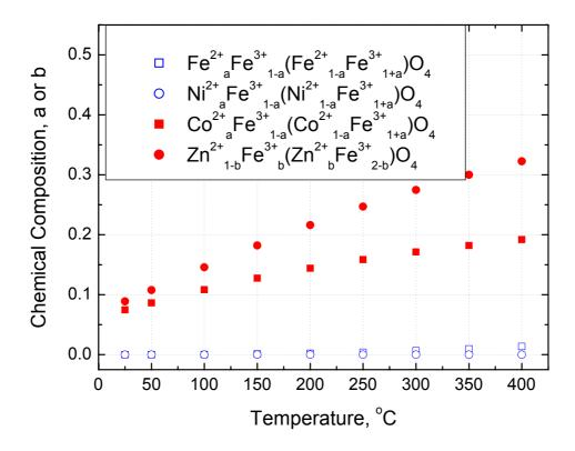
Fig. 4 Cation distribution with temperature in some spinel compounds
