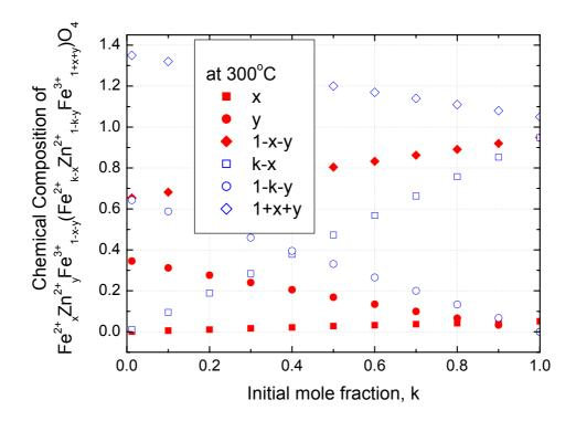
Fig. 12 The values of chemical composition, x+y, 1-x-y and 1+x+y, of  $Fe^{2^+}_{\ x}Zn^{2^+}_{\ y}Fe^{3^+}_{\ 1-x-y}(Fe^{2^+}_{\ k-x}Zn^{2^+}_{\ 1-k-y}Fe^{3^+}_{\ 1+x+y})O_4 \ \ varied \ \ with \ \ initial mole fraction k at 300 °C$
