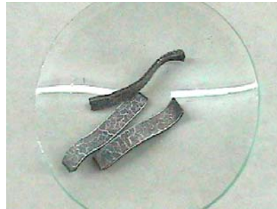
Figure 5. Mini-plates calcined at 700°C in air
