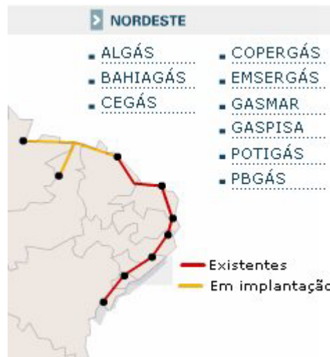
Figure 9. Northeast Gas Pipelines (existing shown in red, in construction shown in orange).
