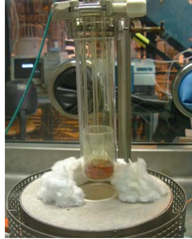
Figure 1: Lab-scale chlorinator in molten chloride bath.
