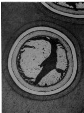
Fig.3 Particle irradiated in FRJ2 reactor (~120 \mu\text{g} Pu/particle, 180 GWd/tM)
