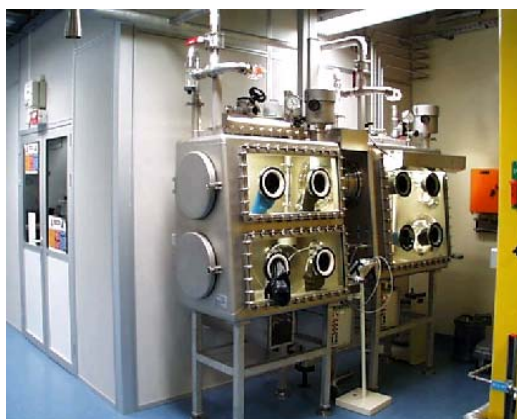
Figure 2: Glove boxes dedicated to the preparation of NMR liquid samples
