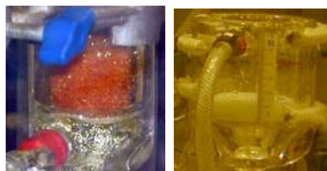
Fig.4. Crystals Obtained in Test (ii) left: U+Pu(VI) right: U+Pu(IV), through lead glass
