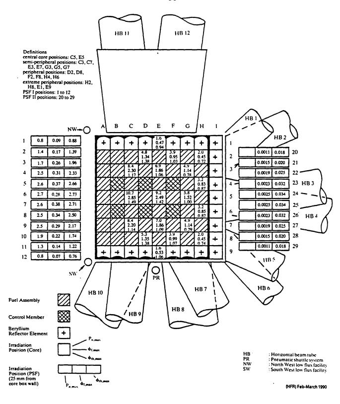
Fig. 3. Standard core configuration with nuclear values and permanently installed experimental reactor facilities
