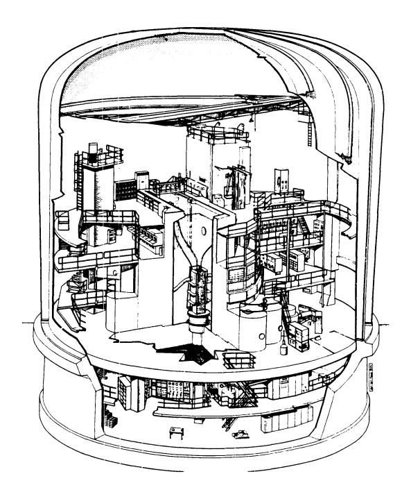
Fig. 2. Isometric drawing of the reactor building
