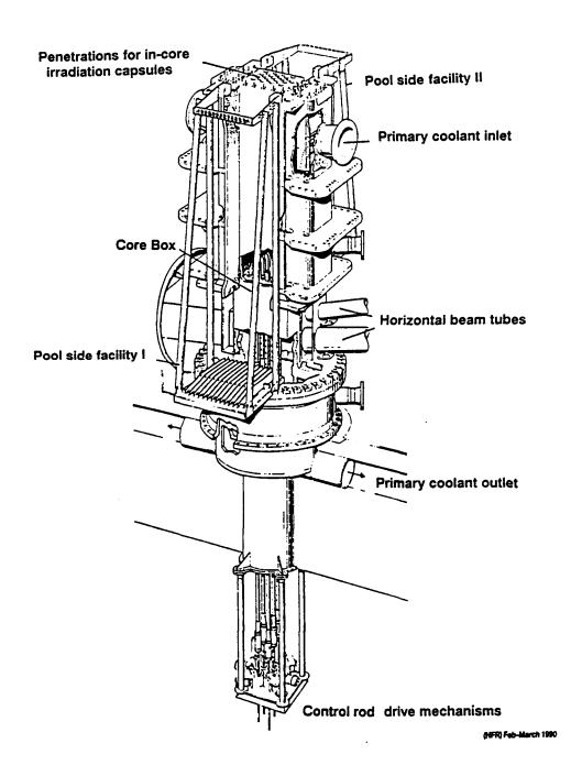
Fig. 1. New reactor vessel of HFR
