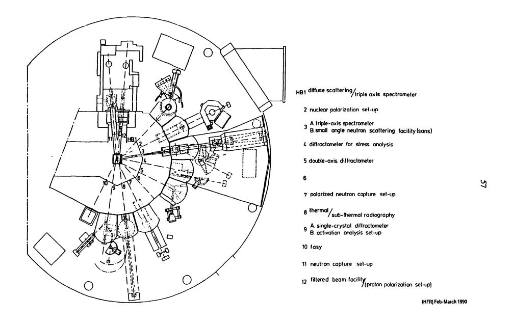
Fig. 4. Horizontal beam-hole neutron experiments
