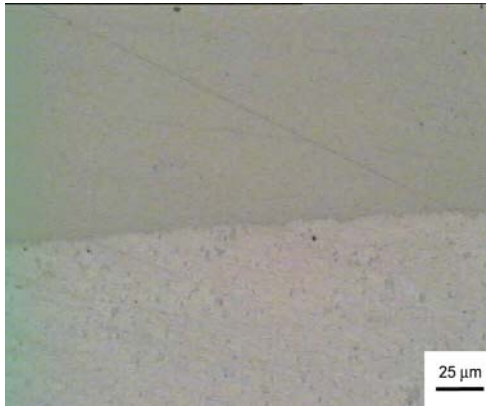
Fig. 2 Welded interface for SS encased in Al. Mechanical polishing up to 1 \mu\text{m} .
